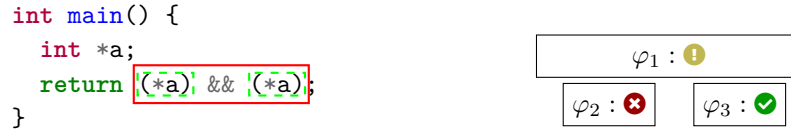
■ Figure 7 Example of different range conventions. In the code, the red rectangle represents a per-statement range and the green dashed rectangles represent per-expression ranges. Then, if analyzer a_1 reports on the entire range, but a_2 reports on the two subexpressions separately, we need to aggregate the results; here, the analyzers are effectively in agreement.
